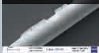
E-Glass in 10% HCl@96C after 24 hours
